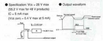
Note: The output waveform for type SQ (R) will be reversed.
