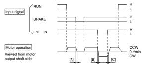
[Notes for "BRAKE" operation and during the rotation direction changing] "BRAKE" (Above [A] period) should be operated, within the "SPEED CONTROL RANGE".
