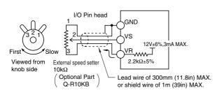
Fig.2 Speed setting by external voltage supply
