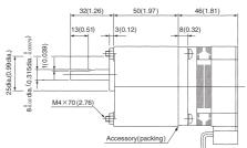
Gearhead weight 0.5Kg(1.1Lb) Bolts (accessory) M4×70(2.76)
