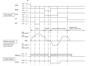
The INT signal is the signal that switches internal speed specified voltage and external speed specified voltage.
